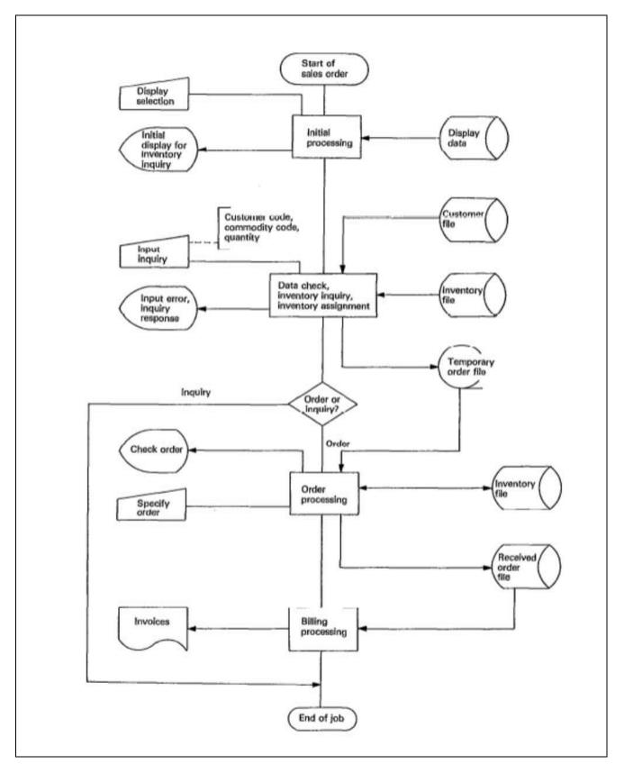
Figure 2: System Flowchart, from ISO 5087, Annex C
